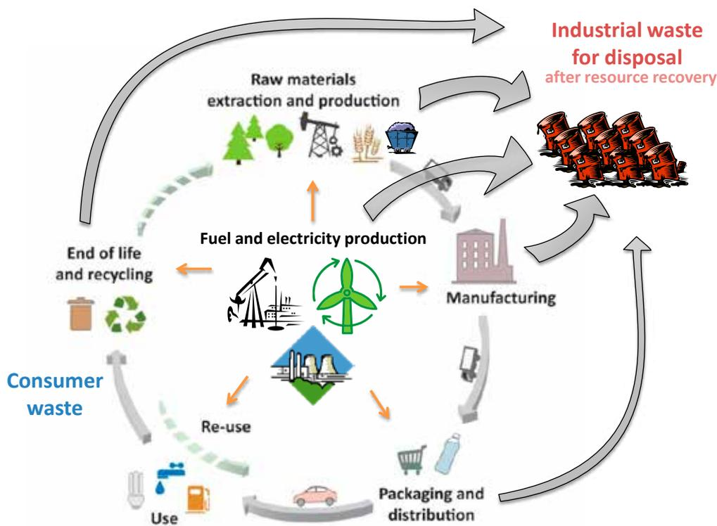
Figure 1 - Life cycle stages of a product and waste generated. Grey arrows represent flows of materials; orange arrows represent energy flows; flows recovered onsite are omitted
